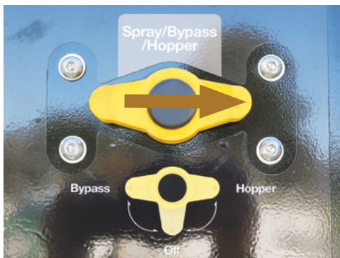
Turn the 'Spray/Bypass/Hopper' valve to Hopper position.
