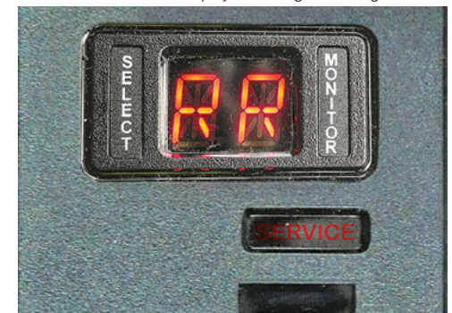
Select & Monitor displays showing Reverse gear.
