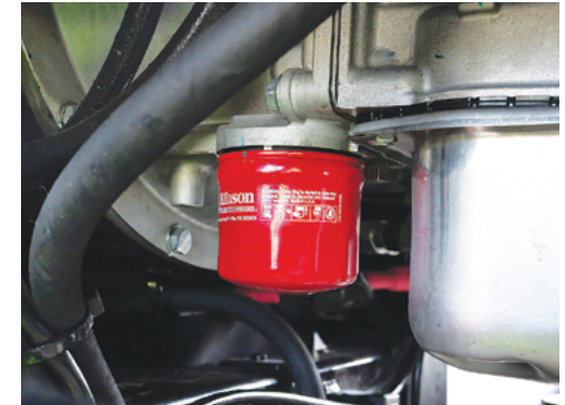
Transmission oil filter.
