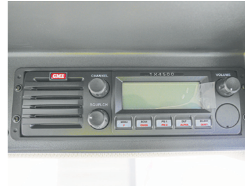
The UHF Two Way Radio located in the Overhead Console above & in front of the operator in the cabin.
