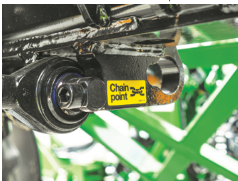
Rear left tie-down attachment point.
