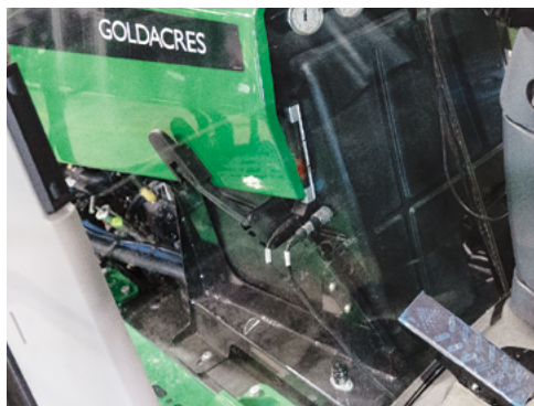
Unclip the bonnet latch located on the left hand side near the cabin.
