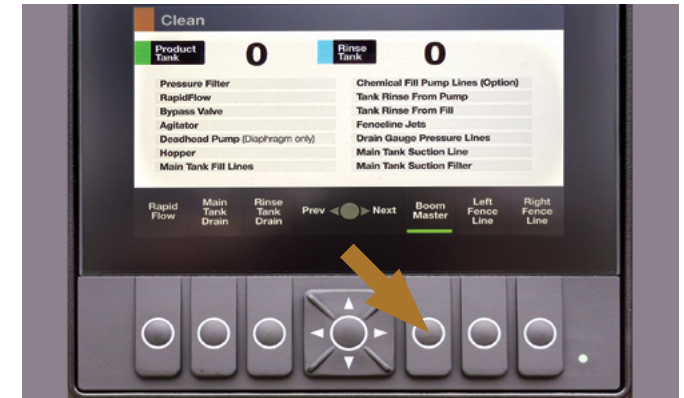
Press the 'Master Switch' push button 'On' to begin rinsing the boom nozzles.
