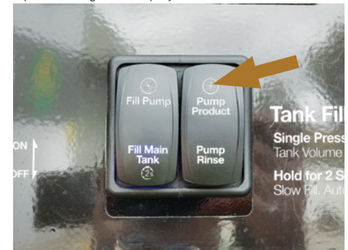
Press-in the 'Pump Product' switch to start pumping product & agitate the spray mixture in the Product tank.
