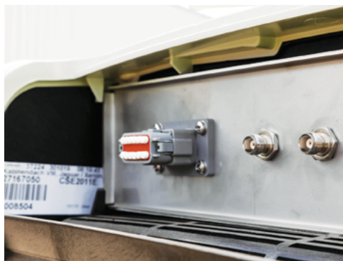
The cover removed showing the antenna connectors.
