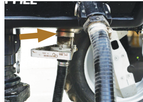
Connect the Micromatic hose to the Crop Cruiser Micromatic rinse coupling outlet for rinsing.
