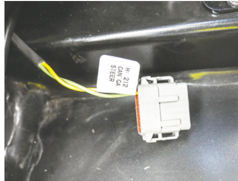
Steering CAN connector in the electrical compartment.
