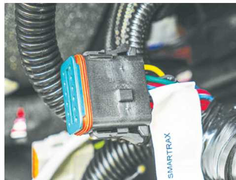
SMARTRAX connector - ISO BUS connection point.
