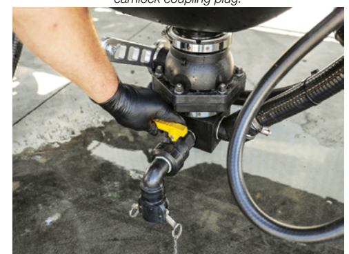
Ensure the Bottom Drain valve is closed & remove the camlock coupling plug.
