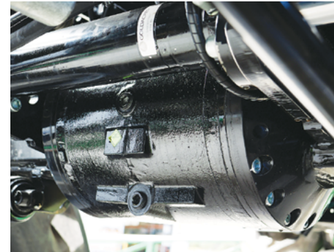
Differential oil drain & fill/oil level plugs.
