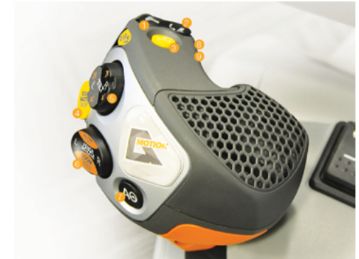
Check all joystick boom switch functions.
