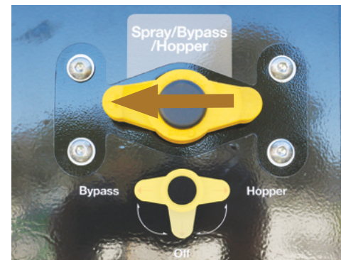
Rotate the 'Spray/Bypass/Hopper' valve to 'Bypass'
