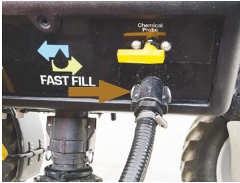
Connect a chemical probe suction hose to the Chemical Probe inlet.
