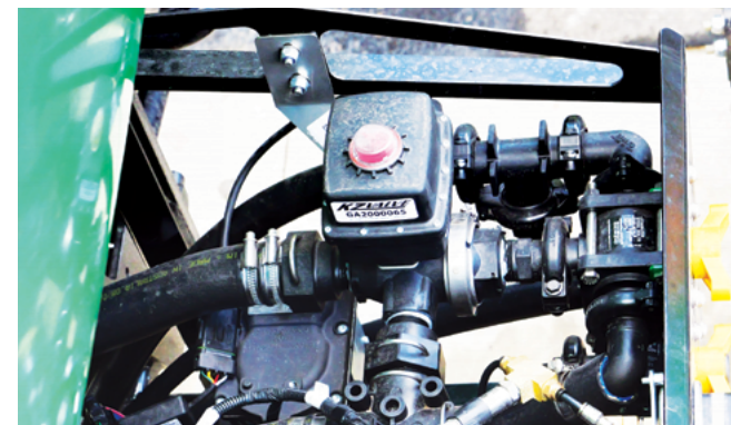
The Regulator Valve, located behind the Quick Fill panel, should regularly be checked & calibrated.
