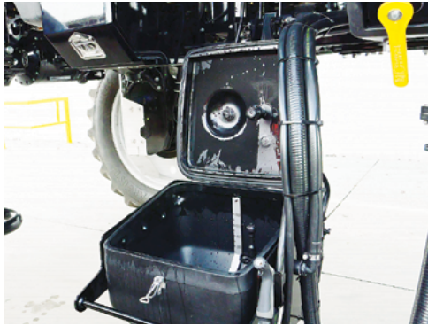
Undo the latch & open the Hopper lid.
