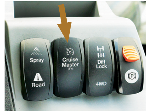
Press the top of the Cruise Master switch to activate or deactivate Cruise Control.
