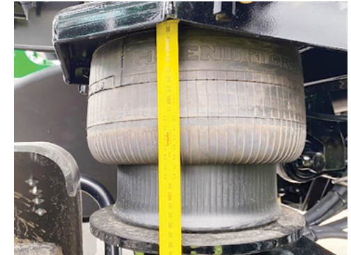
250mm Air bag ride height measurement.
