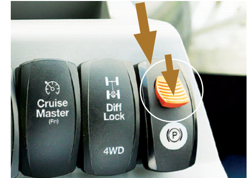
To engage the Park Brake (On), slide the orange lock rearward & press the top of the switch.
