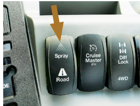
Press the top of the Spray Mode/Road Mode switch to activate Spray Mode
