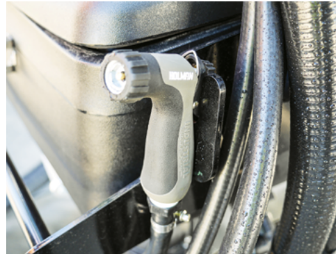
Lift & remove the Wash Down Handgun from its holder on the side of the hopper.
