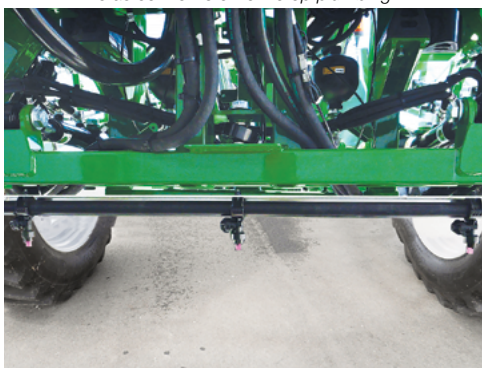
A single nozzle plumbed to the centre of the boom - referred to as centreline or row crop plumbing.
