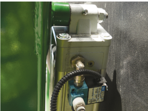
Air inlet of the ladder folding cylinder.
