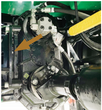
The transfer case oil level plug located on the side of the case.
