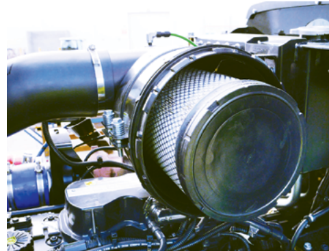
Release the cover from the air cleaner, then remove the primary and secondary filters.
