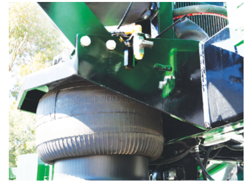
Airbag component of the 5 point suspension system.
