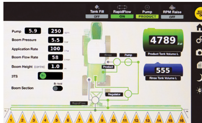
G-Hub Home screen with RapidFlow PRIME completed & the Master Switch On for spraying (Fenceline nozzles Off).
