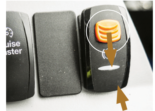
Disengage the Park Brake - slide back the orange lock, then press the switch rearward (Off position).
