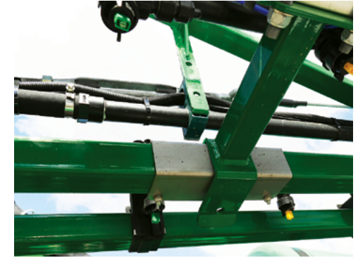
The outer boom rest protection plate must be correctly positioned on each side.
