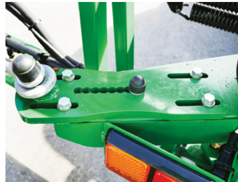
LHS Cable Adjustment Plate.
