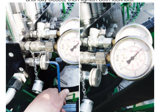
Close (wind-in [clockwise]) both 'Yaw A' & 'Yaw B' valves until fully closed, then tighten both locknuts.
