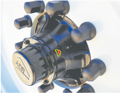
Recommended wheel nut torque tension is 320 ft/lb.
