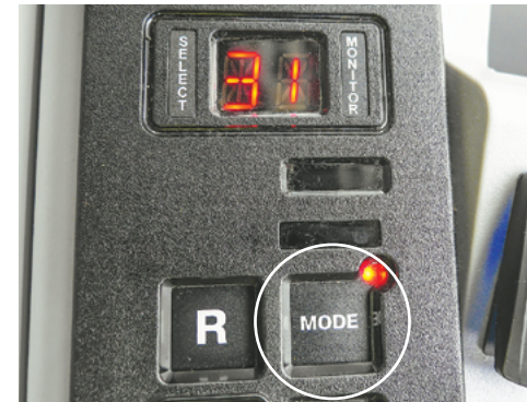
Press the 'Mode' push button to engage the Pre-Select 3rd Gear.
