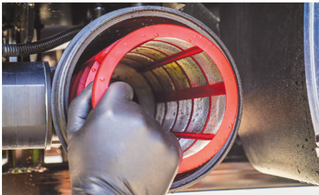
Remove the Suction Filter screen.
